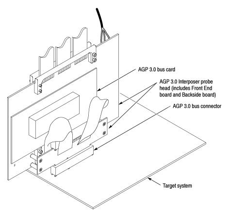
Figure 1-3: Connect the Interposer probe adapter to the AGP 3.0 bus connector
