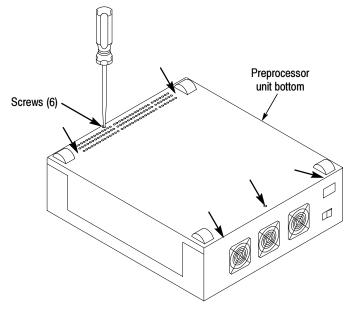
Figure 5-2: Remove the attaching screws
