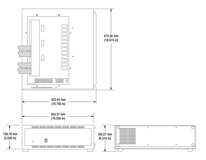
Figure 4-6: Dimensions of the preprocessor unit
