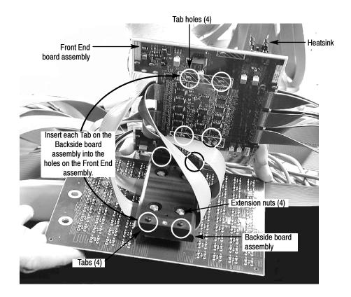
Figure 1-7: Attaching the Front End board assembly
