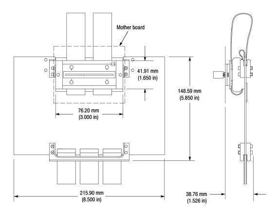
Figure 4-5 shows the dimensions of the AGP 3.0 Backside probe head.
