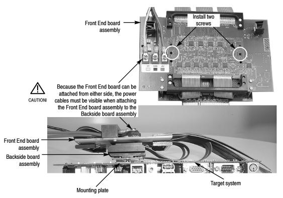
Figure 1-8: Assembled Backside probe head
