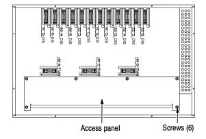
Figure 1-4: Preprocessor unit and access panel
