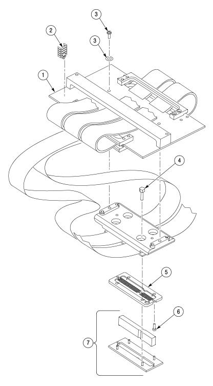
Figure 6-2: Backside probe head exploded view
