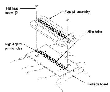
Figure 1-15: Replacing the Pogo pin assembly on the Backside board
