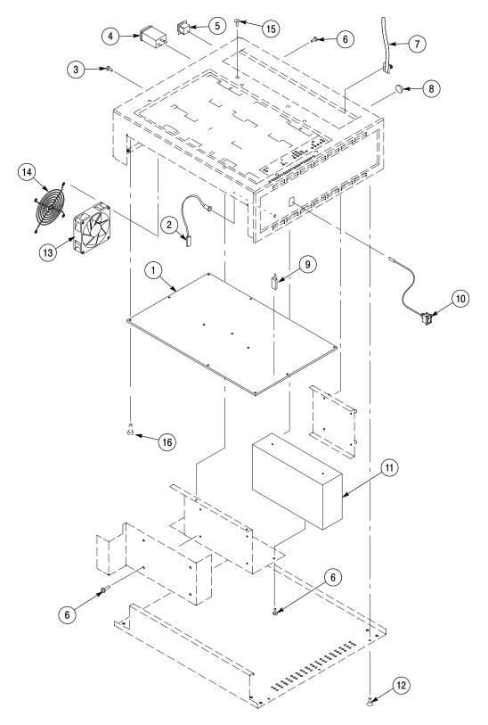
Figure 6-3: Preprocessor unit exploded view
