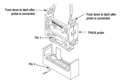
Figure 1-12: Operating the P6434 probe latches
