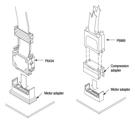
Figure 1-13: Probes with mictor adapters
