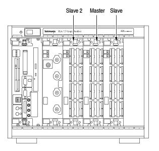
Figure 3-1: Configuration for slave 2, master, and slave modules
