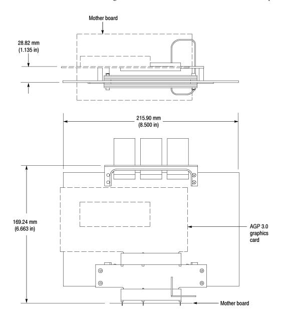
**Dimensions** Figure 4-4 shows the dimensions of the AGP 3.0 Interposer probe head.
