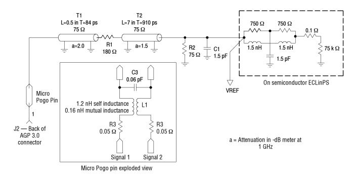
Figure 4-3: Backside source sync load model
