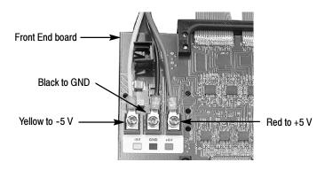
Figure 1-9: Attach the power cables
